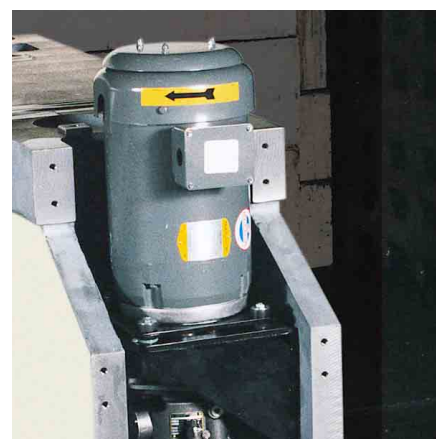
Hydraulic motor pump assembly mounted in left hand rear press bed leg.
